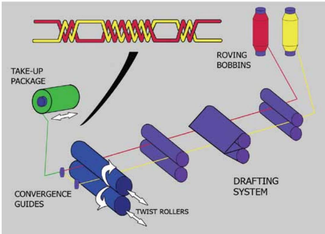
The eco-SpinTwist offers spinning and twisting on one machine.
